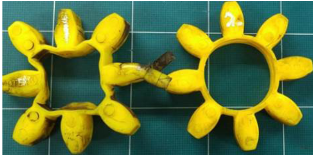
Fig. 1: A worn spider next to a new one
